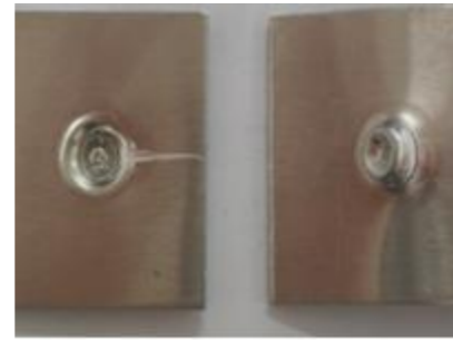
接头失效 joint failure
